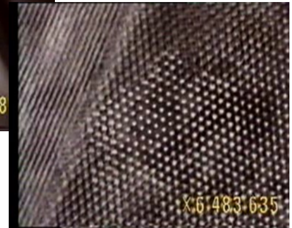
Structure atomique \text{Al}_2\text{O}_3 (0.1 nm)
